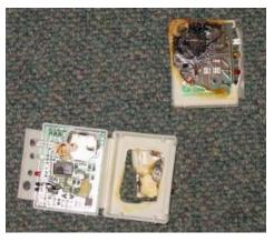
Figure 16 Damaged Lighting Loggers
