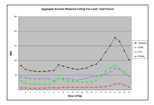
Figure 25 Summer Weekend Ceiling Fan Total Fixture System Load
