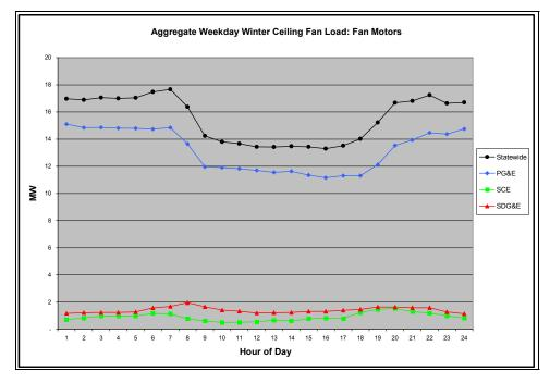
Figure 35 Winter Weekday Ceiling Fan Motor System Load
