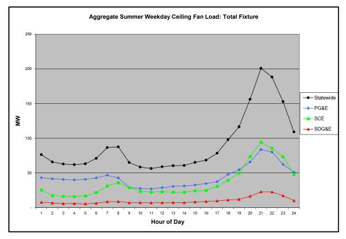
Figure 22 Summer Weekday Ceiling Fan Total Fixture System Load
